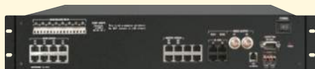
AX-084C Central Exchange Unit (supports up to 4 master stations and 8 door/sub stations)
